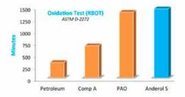
The primary cause of degradation is oxidation. S-Series is much more oxidation-resistant than petroleum oils.\*\*
