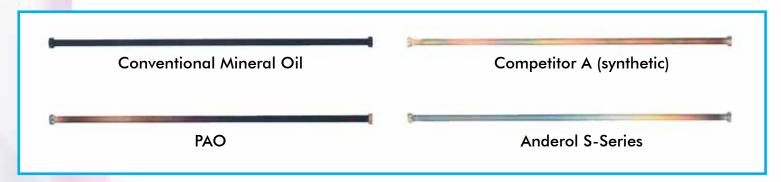
Our advanced lubrication and additive technology has enabled us to create a unique product that rivals the qualities of jet turbine lubricants. The highly sophisticated High Temperature Deposition Test is required for military and civilian jet oils around the world; the better the lubricant, the smaller the amount of lacquer deposited on the steel rods. Note that the rod testing S-Series Lubricant is almost totally clean!
