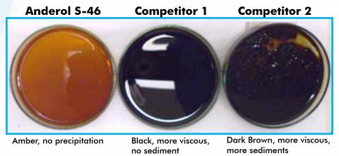
Dramatic color changes were observed in both competitors samples within the first  $\frac{1}{2}$  hour of analysis. This continued for both the competitors samples 1 and 2, throughout the 12-hour testing period. In the 8-hour and 12-hour period a more viscous sample with sediments was observed in the Competitor 2 sample. For the competitor 1 sample in the 12-hour period a color change was observed from Dark Brown to Black.
