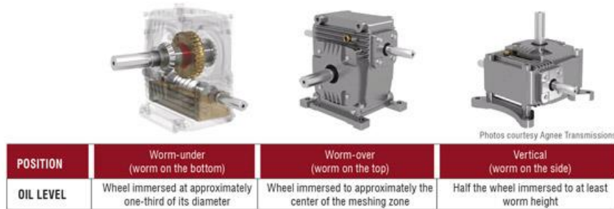
Figure 10. The three most common worm drive positions (Ref: The Lubrication Engineers Manual )
